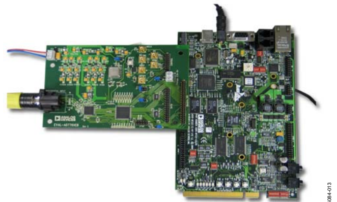
Figure 13. Powered Up AD7764/AD7765 Evaluation Kit
