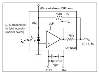
FIGURE 1. Basic Circuit Connections.
