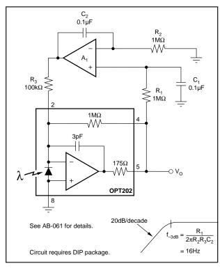
FIGURE 8. DC Restoration Rejects Unwanted Steady-State Background Light.
