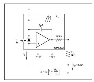
FIGURE 6. Current Output Circuit.
