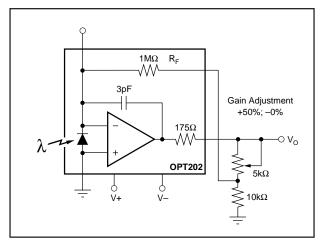
FIGURE 4. Responsivity (Gain) Adjustment Circuit.
