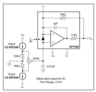
FIGURE 3. Dark Error (Offset) Adjustment Circuit.
