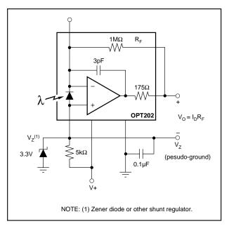
FIGURE 7. Single Power Supply Operation.
