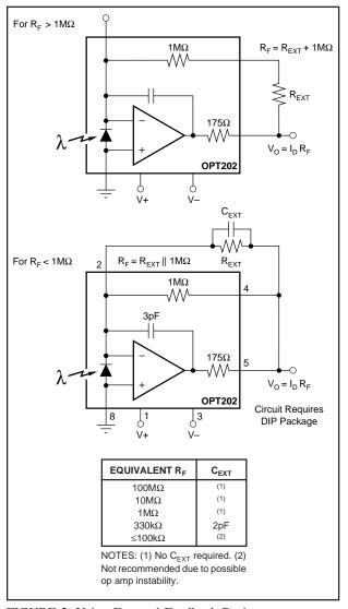
FIGURE 2. Using External Feedback Resistor.
