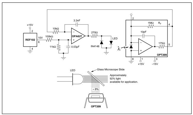
FIGURE 12. LED Output Regulation Circuit.
