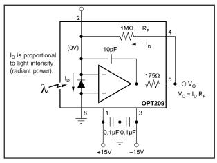
FIGURE 1. Basic Circuit Connections.
