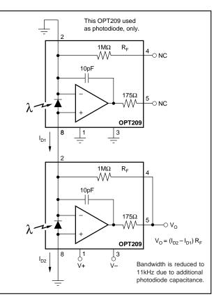
FIGURE 7. Differential Light Measurement.
