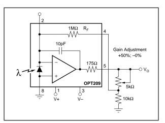
FIGURE 4. Responsivity (Gain) Adjustment Circuit.
