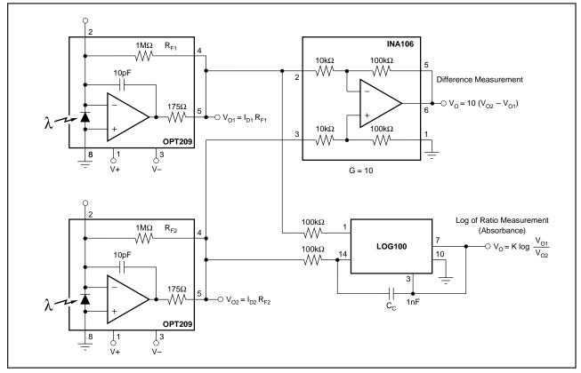
FIGURE 11. Differential Light Measurement.
