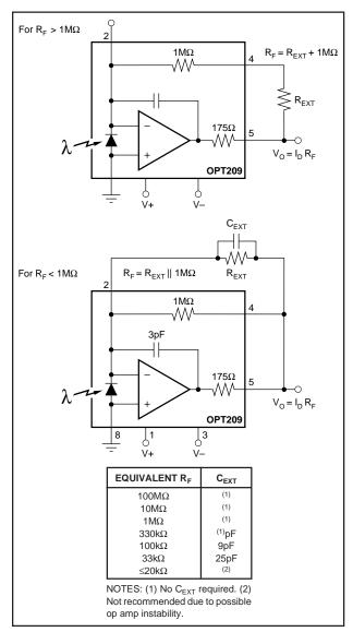
FIGURE 2. Using External Feedback Resistor.
