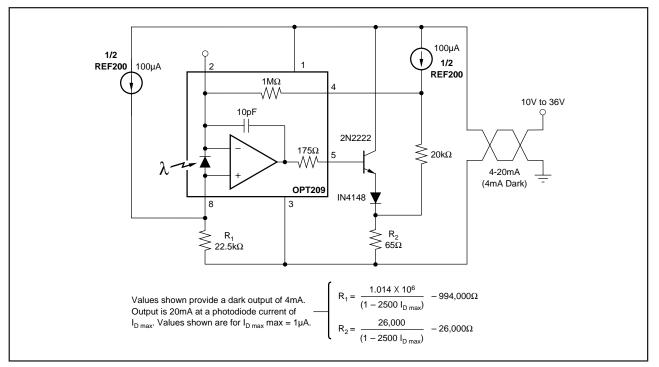
FIGURE 13. 4-20mA Current-Loop Transmitter.
