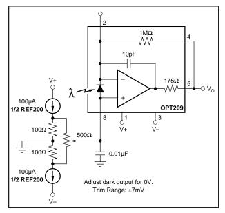
FIGURE 3. Dark Error (Offset) Adjustment Circuit.
