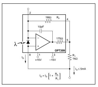
FIGURE 8. Current Output Circuit.
