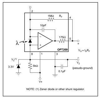
FIGURE 9. Single Power Supply Operation.
