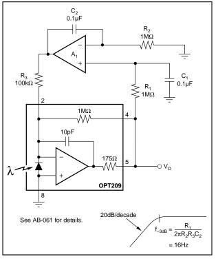
FIGURE 10. DC Restoration Rejects Unwanted Steady-State Background Light.
