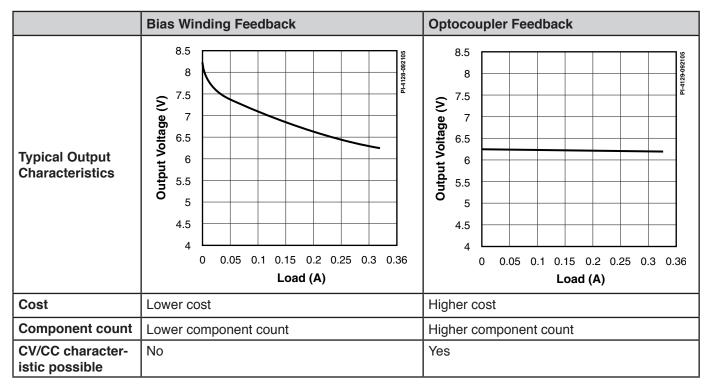
Table 3. Summary of Comparison Between Bias Winding Feedback and Optocoupler Feedback.
