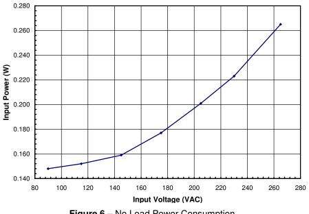
Figure 6 – No Load Power Consumption.
