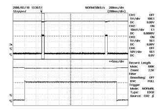
Figure 17 – Transient Response, 265 VAC. Upper: V<sub>OUT</sub>, 5 V / div. Lower: I<sub>OUT</sub>, 1.0 A / div. Timebase: 200 ms / div.
