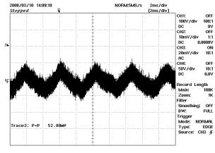
Figure 28 - Ripple, 265 VAC, 35 W Load. 20 mV / div, 2 ms / div.
