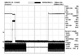
Figure 21 – AC Reset, 265 VAC. Upper: V<sub>OUT</sub>, 5 V / div. Middle: I<sub>OUT</sub>, 1.0 A / div. Lower: AC Input, 500 V / div. Timebase: 500 ms / div.
