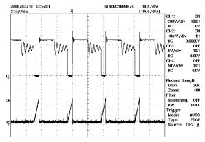
Figure 11 – 265 VAC, 35 W Load. Upper:  $V_{DRAIN}$ , 200 V / div. Lower:  $I_{DRAIN}$ , 0.5 A / div. Timebase: 10  $\mu$ s / div.
