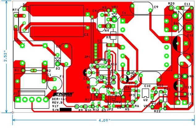
**Figure 3** – Printed Circuit Layout.
