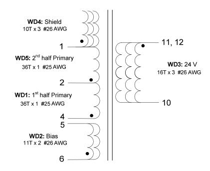
Figure 4 – Transformer Electrical Diagram.
