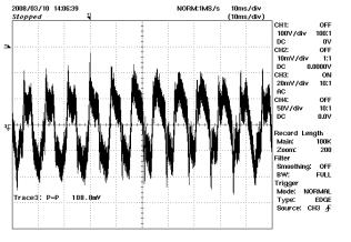
Figure 27 – Ripple, 90 VAC, 35 W Load. 20 mV / div, 10 ms / div.
