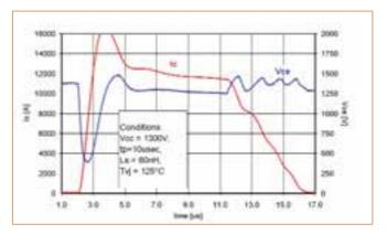
Figure 4b. SCSOA 3600A/1700V HiPak switching characteristics under SOA conditions at 125°C.
