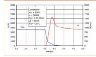
Figure 3a. Turn-on waveforms 3600A/1700V HiPak switching characteristics at 125°C.
