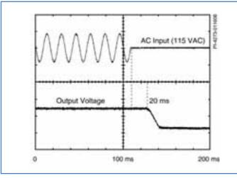
Figure 5. Comparison of a design with and without the on-time extension feature, showing 20% improvement in hold-up time.
