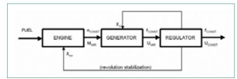
Figure 2. Concept EGS with constant speed of engine.
