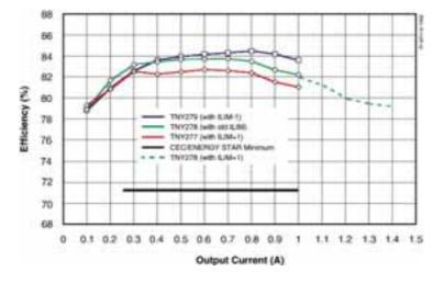
Figure 4.Trade off between device size, current limit, efficiency and power delivery.
