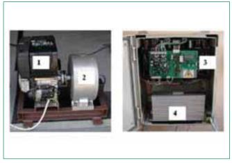
Figure 5. The photo of experimental model (1-diesel engine; 2-SGPM; 3- AC/DC/AC converter; 4-filter).
