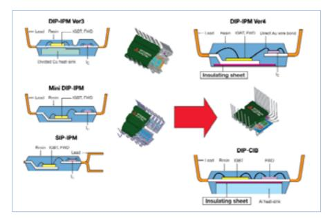
Figure 7. Trends in Package Structures of DIP-IPM.
