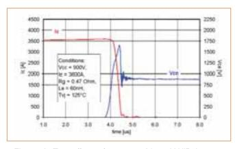
Figure 3b. Turn-off waveforms 3600A/1700V HiPak switching characteristics at 125°C.
