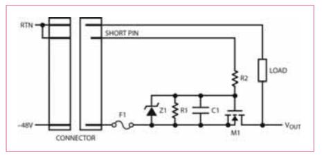
Figure 1. A passive hot swap circuit softens the connection of power to a card.
