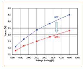
Figure 2. SPT and SPT<sup>+</sup> IGBT on-state voltage vs. rated blocking voltage at 125°C.
