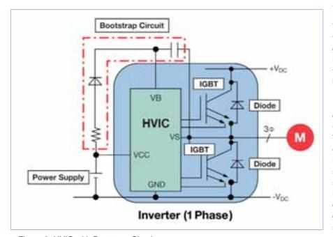
Figure 3. HVIC with Bootstrap Circuit.
