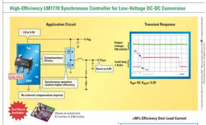
The LM1770 is simple to use and provides higher efficiency than LDOs.
