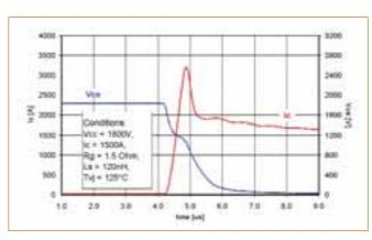
Figure 5a. Turn-on waveforms 1500A/3300V HiPak switching characteristics at 125°C.
