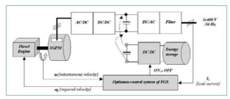
Figure 10. The EGS system with peak power energy to DC link of AC/DC/AC converter.
