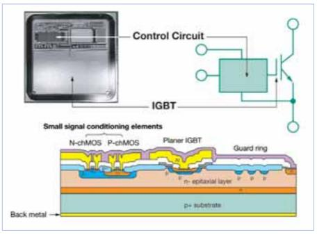
Figure 4. Top View and Structure of Intelligent Power Device.
