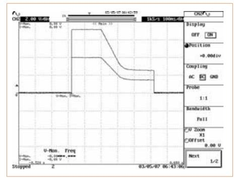
Figure 2. For safe operation, the curve of overload performance must be investigated in every case. After 200ms of a 3-phase overcurrent the power amplifier automatically reverts to the nominal value.
