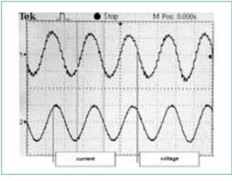
Figure 7. Output voltage and current of EGS.
