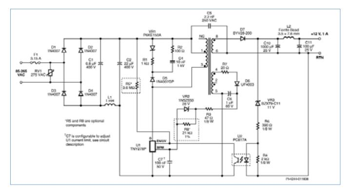
Figure 2. TinySwitch-III schematic implementing a 12 V, 1 A design.
