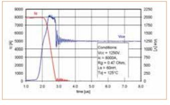
Figure 4a. RBSOA 3600A/1700V HiPak switching characteristics under SOA conditions at 125°C.
