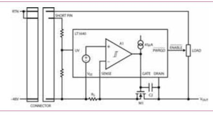
Figure 2. Early hot swap controllers limit inrush current more accurately, turn off faster when disconnecting, and include an electronic circuit breaker.
