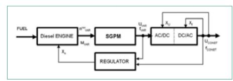
Figure. 3. The concept EGS with optimum variable speeds according load.
