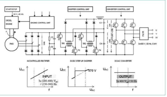
Figure 6. The schematic circuit of experimental model with AC/DC/AC converter.
