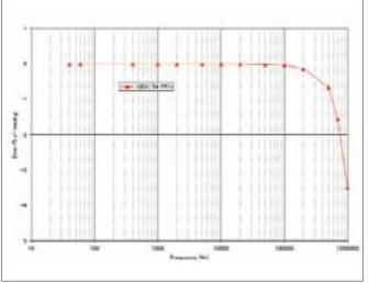
Figure 4. Power error curve with respect to frequency.
