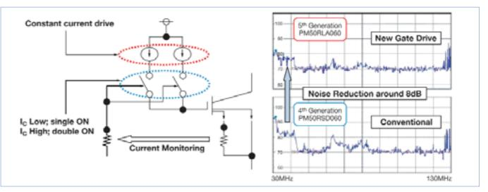
Figure 1. New Gate Drive Concept to Reduce Switching Noise.
