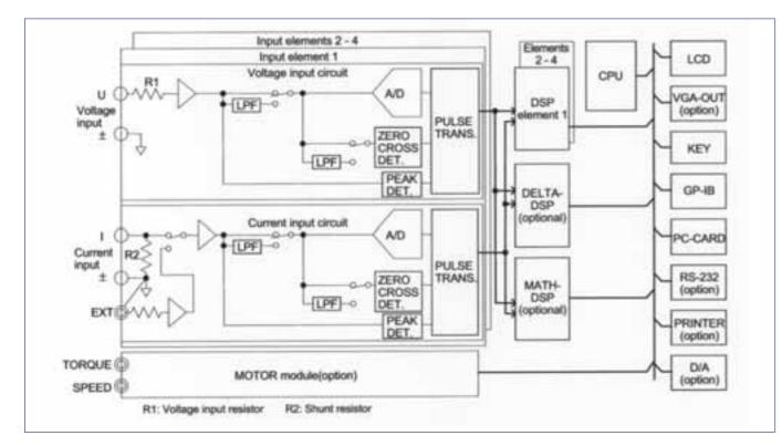
Figure 2. Schematic of the WT3000 precision power meter.
