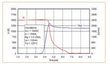
Figure 5b. Turn-off waveforms 1500A/3300V HiPak switching characteristics at 125°C.
