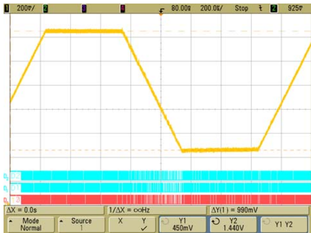
Figure 8. DVID Waveform (by VTT, 0.5 V-1.5V) 1-Vo D0~D2-PWM1~3
