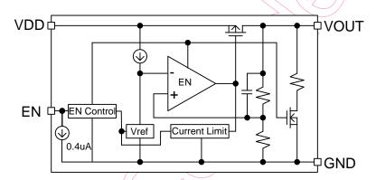
Figure 2(a) Functional diagram of Fix mode
