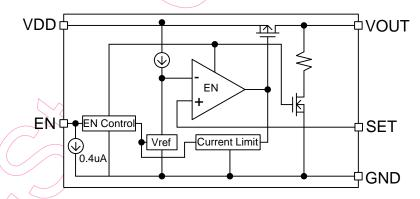
Figure 2(b) Functional diagram of Adjustable mode
