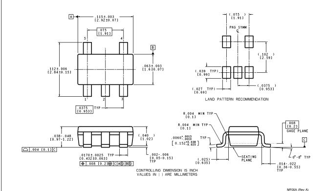
5-Lead SOT-23 Package Order Number LM2733XMF, LM2733XMFX, LM2733YMF or LM2733YMFX **NS Package Number MF05A**
