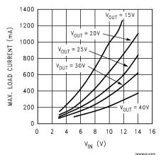
LM2733y Max. Load Current vs V<sub>IN</sub>
