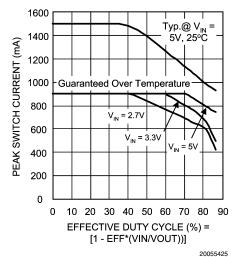
LM2733x Switch Current Limit vs Duty Cycle
