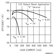
$\begin{tabular}{ll} \textbf{Typical Performance Characteristics} & \textbf{Unless otherwise specified:} & \textbf{T}_{A} = 25 ^{\circ} \textbf{C}, & \textbf{C}_{OUT} = 4.7 ~\mu \textbf{F}, & \textbf{C}_{IN} = 2.2 ~\mu \textbf{F}, & \textbf{SHDN pin is tied to V}_{IN}, & \textbf{V}_{IN} = 5 \textbf{V}, & \textbf{LM2733X}, & \textbf{L} = 10 ~\mu \textbf{H}. & \textbf{(Continued)} \\ \end{tabular}$
