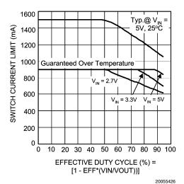
LM2733y Switch Current Limit vs Duty Cycle
