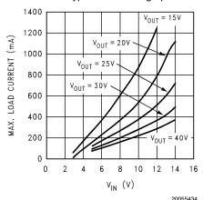
LM2733x Max. Load Current vs VIN
