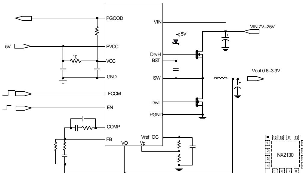
Figure 1 - Typical application of 2130
