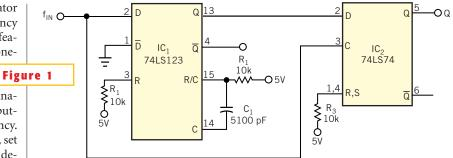
This simple circuit can reveal whether an input frequency is above or below a reference frequency.
