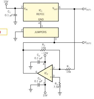
This pin-configurable voltage reference delivers a variety of positive and negative output voltages.
