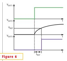
One additional comparator produces a positive signal at the processor's reset port.
