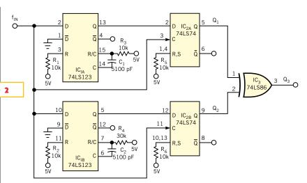
Doubling the circuit in Figure 1 and using an exclusive-OR circuit results in a window discriminator.
