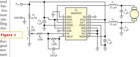
A Class D audio amplifier, IC,, helps implement this simple motor-speed controller.
