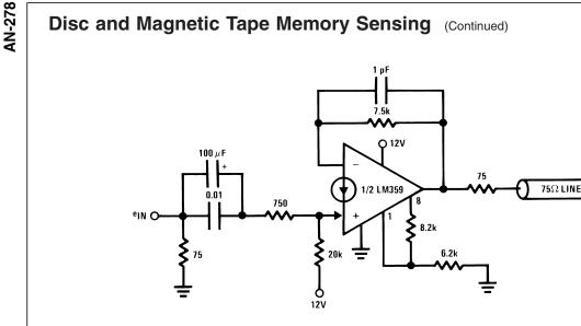
FIGURE 8. A Typical Application of this Fast Norton Amplifier
