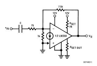
FIGURE 11.  $nV_{BE}$  Biasing Can Reduce Input Noise Voltage
