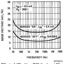
a) Effect of "Shutting Off" the Input Mirror
