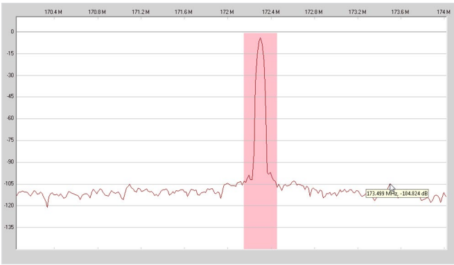
Figure 6. 1.2 MHz sideband switching spur at 170 MHz input. Spur level = -105 dBFS.
