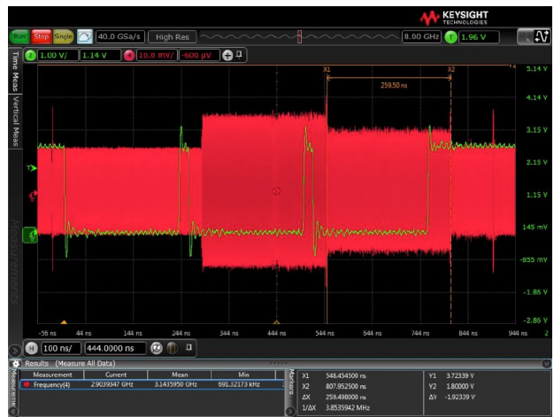
Figure 6. Fast frequency hopping performance of the AD9164—260 ns dwell time per hop.
