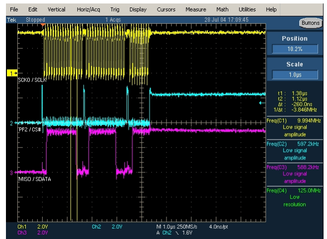
Figure 6. AD7276 Power-Down Mode
