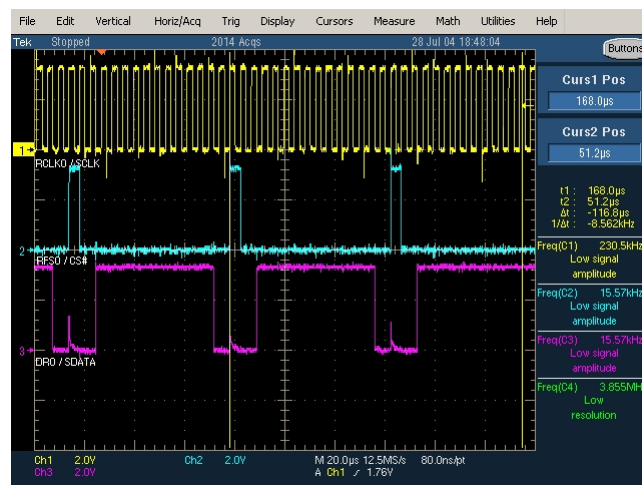
Figure 8. SPORT Early Frame Sync Option, Rising Clock Edge Sampling - Core Mode
