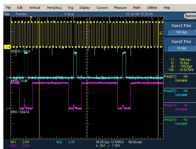
Figure 9. SPORT Late Frame Sync Option, Rising Clock Edge Sampling - Core Mode
