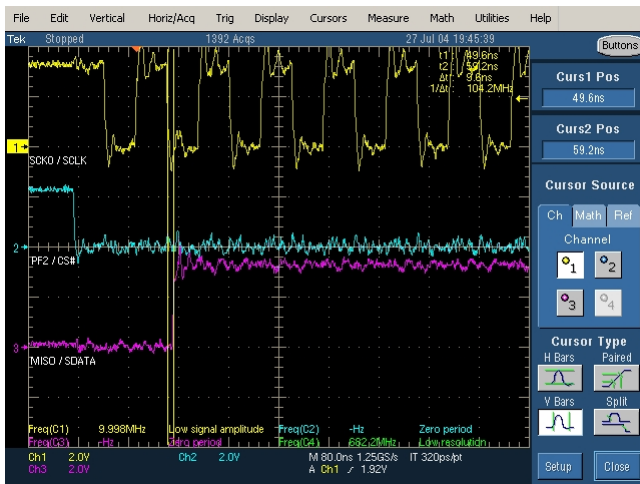
Figure 4. CPHASE=0, CPOL=1 in Core Mode – AD7276 Hold Time
