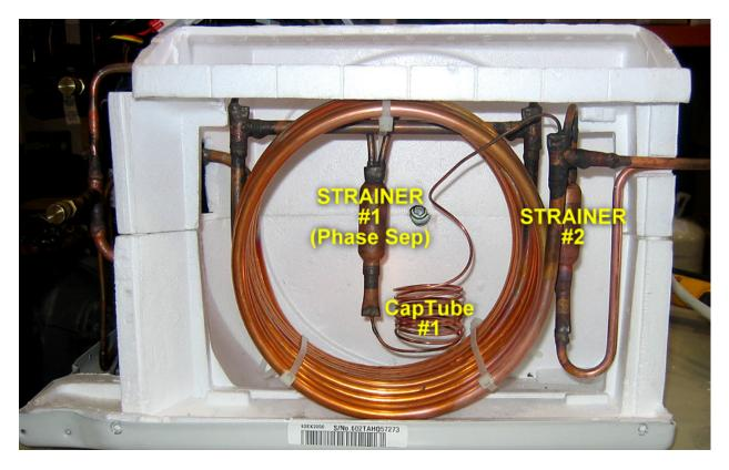
The autocascade heat exchangers reside in the space once occupied by the stock evaporator, and circulation fan. This area will later be insulated with self-expanding polyurethane closed cell foam.
