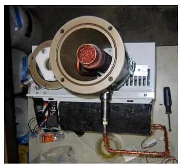
Here's a birds-eye view of the connected cold trap (modified vacuum pump exhaust filter housing). Inside can be seen the evaporator assembly which consists of a 12" length of 1 5/8"od copper tubing with ¼"od tubing coiled around and brazed to its outside surface.
