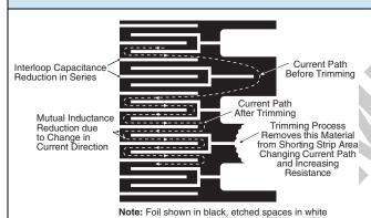
To acquire a precision resistance value, the Bulk Metal<sup>®</sup> Foil chip is trimmed by selectively removing built-in "shorting bars." To increase the resistance in known increments, marked areas are cut, producing progressively smaller increases in resistance. This method reduces the effect of "hot spots" and improves the long term stability of the Vishay Foil chips.
