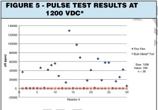
\* Note: Average of 30 units yielded deviation of 30,723 ppm for the Thin Film vs. -14 ppm for the Bulk Metal® Foil
