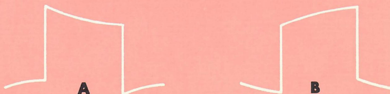
Fig. 6. Illustrating low-frequency defects in square waves. In A, the low-frequency components have leading phase angles and are attenuated. In B, the low-frequency components have lagging phase angles and are accentuated.
