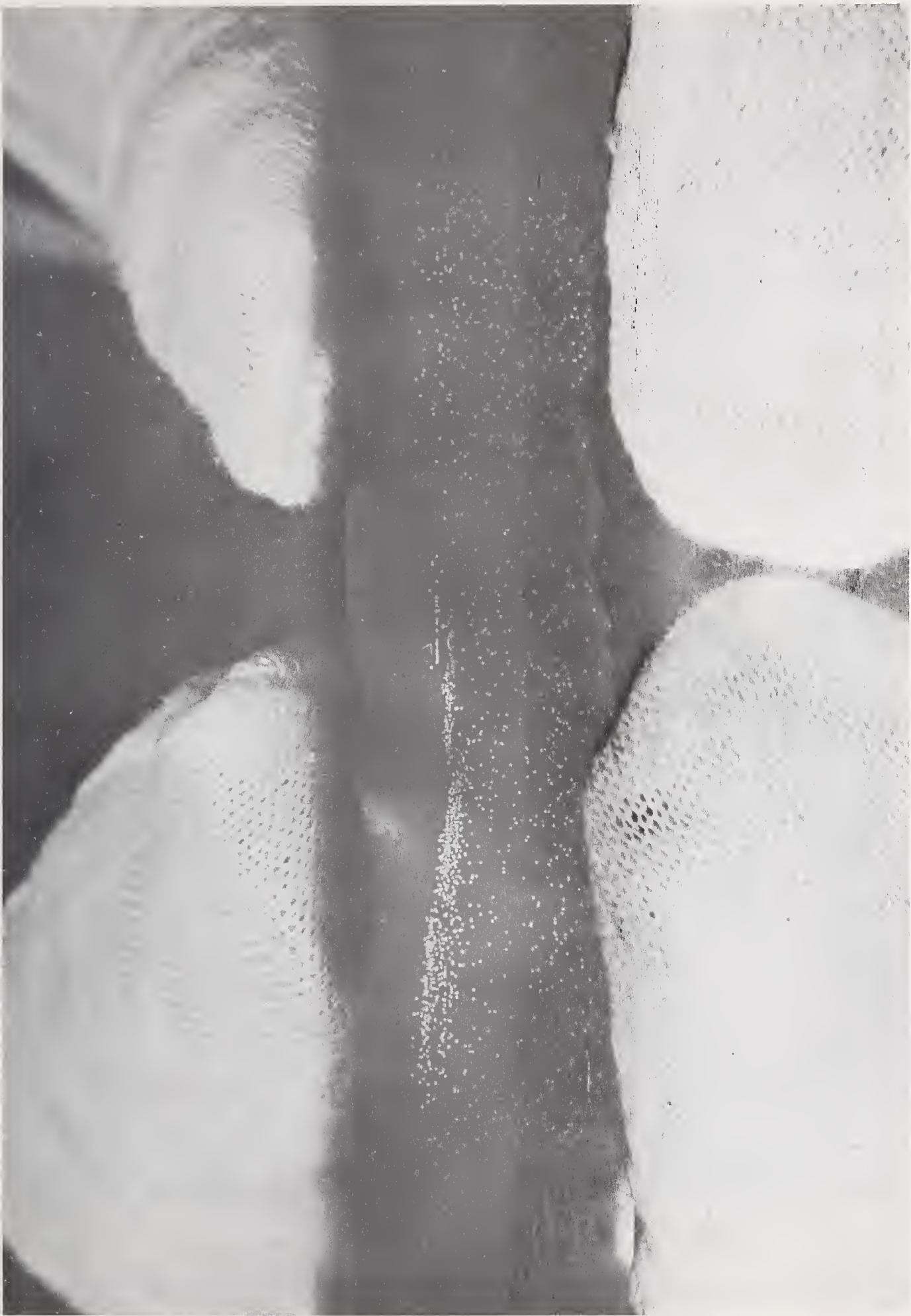
FIGURE 7. Some spots can be seen with the unaided eye. Here the silvery sheen of type 1 is seen on a 16 mm fogged leader by reflected light.
