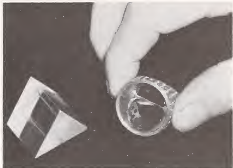
FIGURE 11. Photograph of two Koesters double-image prisms, one mounted in a cell and the other untrimmed.
