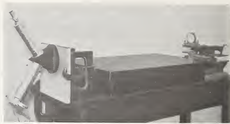
FIGURE 2. Pilot model of surface plate interferometer for testing feasibility of the optical principals with a typical granite surface plate.
