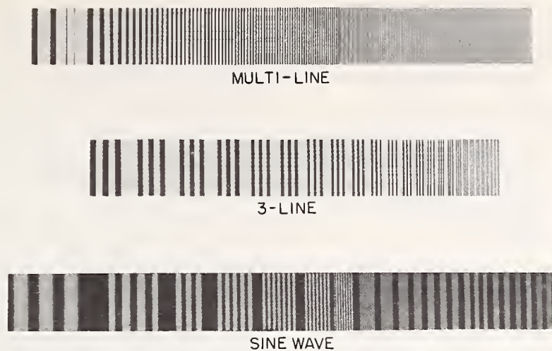
FIG. 1. Three types of resolution targets which have been used to determine image contrast.
