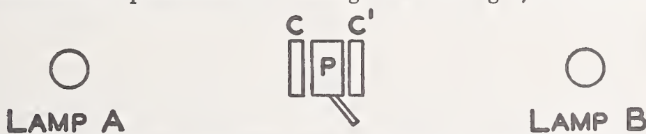
FIGURE 33.—Schematic diagram showing photometer used to test the color match of the lamp-and-filter combinations
