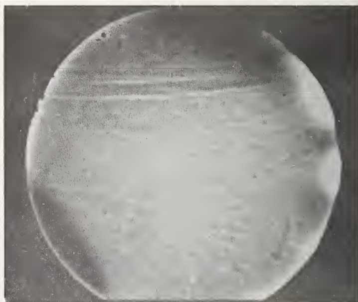
Fig. 8. A shadowgraph of silicon made with an image converter. Horizontal streak in upper half of sample indicates an area of striae.
