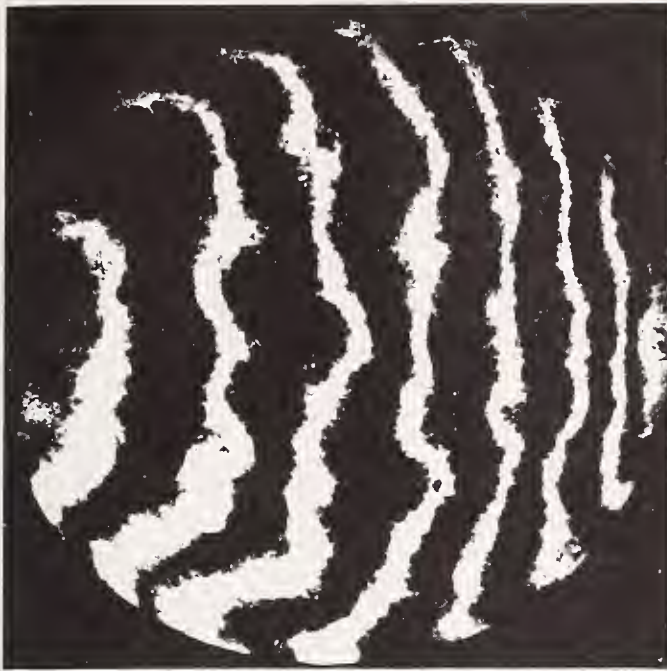
FIGURE 8. Topographic map of one optical surface, relative to a standard, produced by photographing a given fringe (order of interference) successively, as it was moved across the plate, by controlled evacuation of air wedge between the plates.
