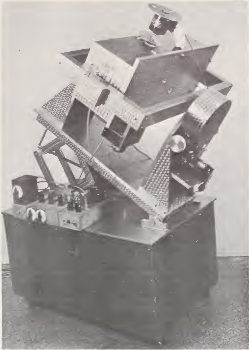
FIG. 21. Photograph of solar spectroradiometer mounted on a polar axis.
