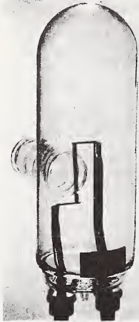
FIGURE 1. Tungsten ribbon strip lamp standard of spectral radiance.
