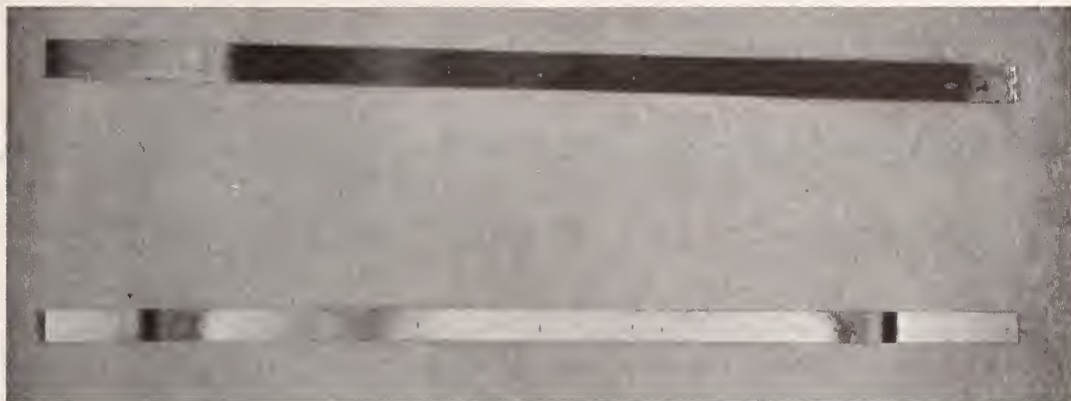
Fig. 6. Strips of Type 430 stainless steel. The dark strip was tested at a maximum temperature of 809°C., and the bright strip was tested at a maximum temperature of 1000°C. The oxide layer that was formed at temperatures in the range of 600–800°C. apparently decomposed or volatilized on heating to 1000°C.
