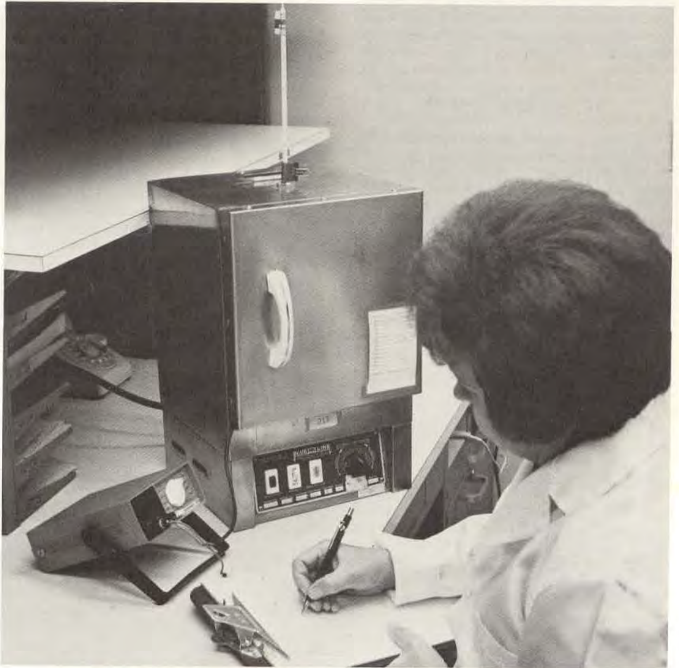
Fig. 2-25 Equipment configuration for temperature coefficient demonstration
