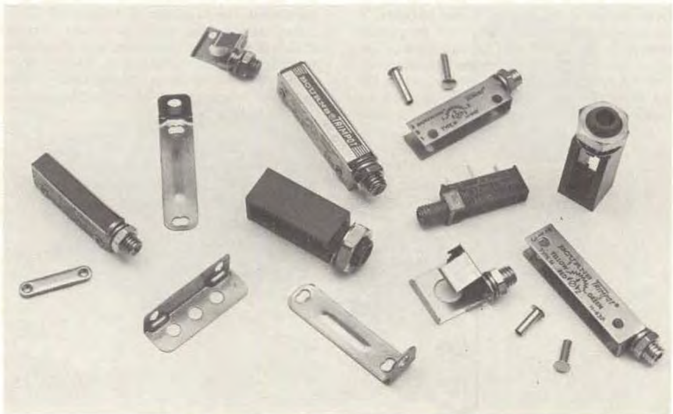
Fig. 8-15 Adjustment potentiometer mounting hardware
