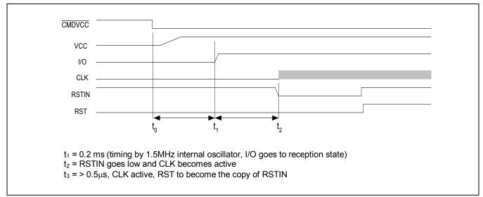
Figure 7: Activation Sequence—RSTIN High When CMDVCC Goes Low
