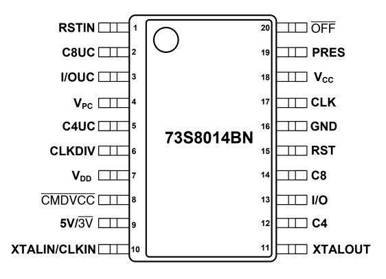
Figure 2: 73S8014BN 20-SO Pinout
