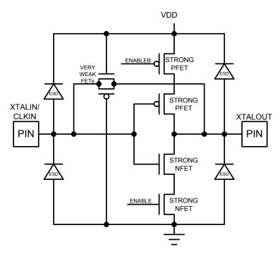
Figure 19: Oscillator Circuit
