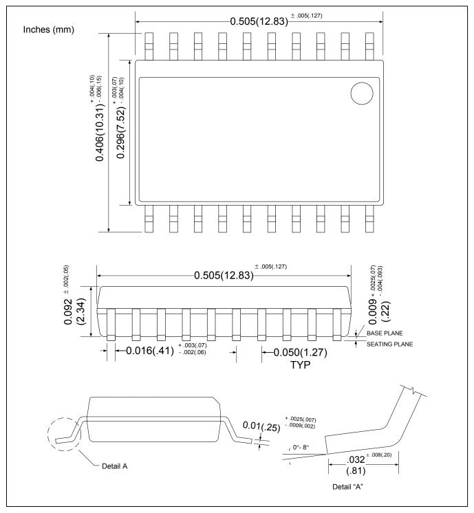
Figure 21: Mechanical Drawing 20-Pin SO Package
