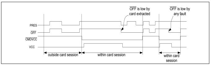
Figure 9: Timing Diagram—Management of the Interrupt Line OFF
