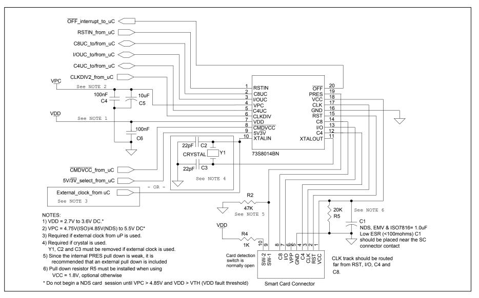
Figure 3: 73S8014BN—Typical Application Schematic
