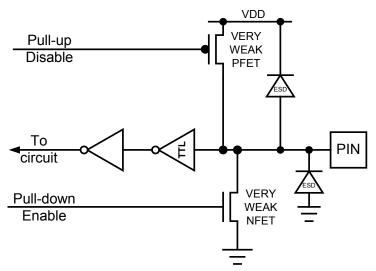
Note:  $5V/\overline{3V}$  has the pullup enabled. PRES has the pulldown enabled. CMDVCC and RSTIN have pullup and pulldown disabled.
