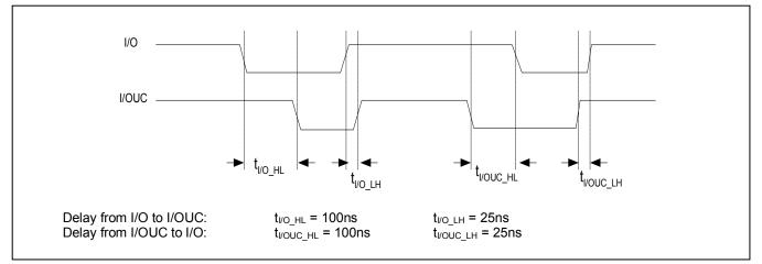
Figure 11: Timing Diagram—I/O to I/OUC Delays
