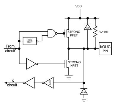
Figure 17: Smart Card I/OUC Interface Circuit
