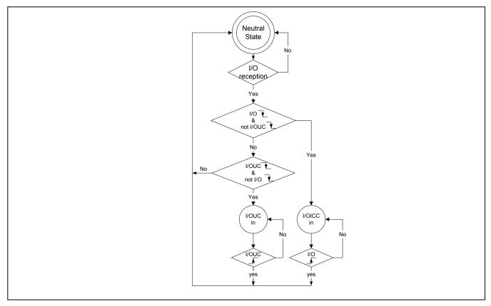
Figure 10: I/O and I/OUC State Diagram
