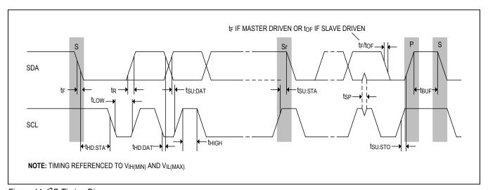
Figure 44: I<sup>2</sup>C Timing Diagram
