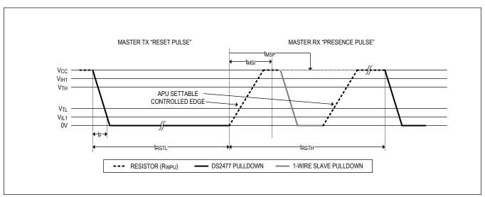
Figure 2. 1-Wire Reset/Presence-Detect Cycle
