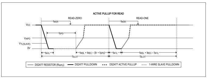
Figure 7. Active Pullup for 1-Wire Read Time Slot
