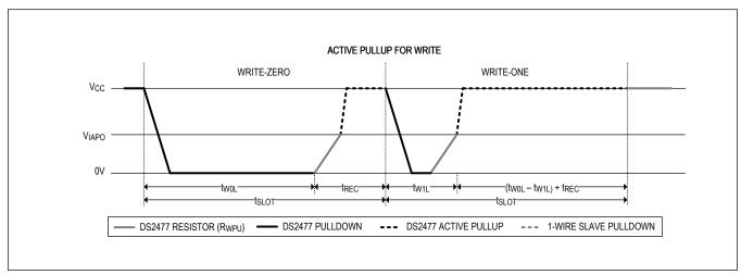
Figure 6. Active Pullup for 1-Wire Write Time Slot
