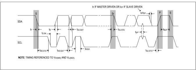
Figure 10. I<sup>2</sup>C Timing Diagram
