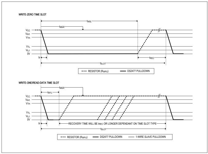
Figure 3. Read/Write Timing Diagrams
