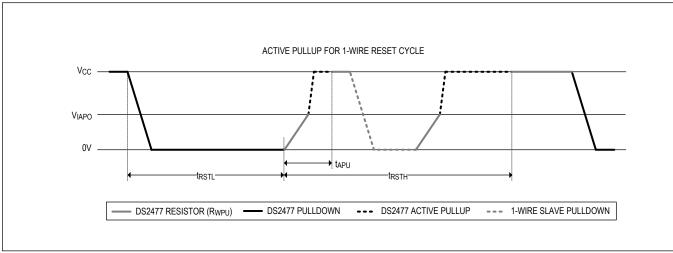
Figure 5. Active Pullup for a 1-Wire Reset Cycle
