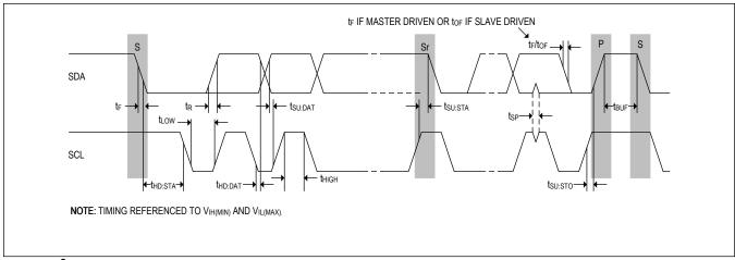
Figure 3. I<sup>2</sup>C Timing Diagram
