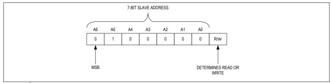
Figure 2. I<sup>2</sup>C Slave Address
