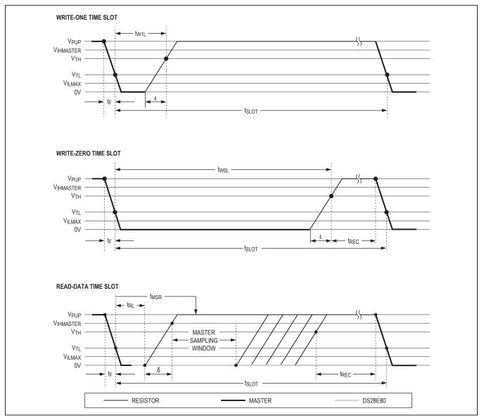
Figure 10. Read/Write Timing Diagram
