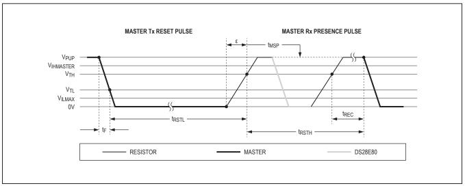
Figure 9. Reset/Presence pulse
