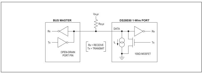
Figure 7. Hardware Configuration
