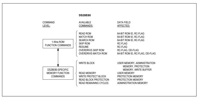
Figure 2. Hierarchical Structure for 1-Wire Protocol
