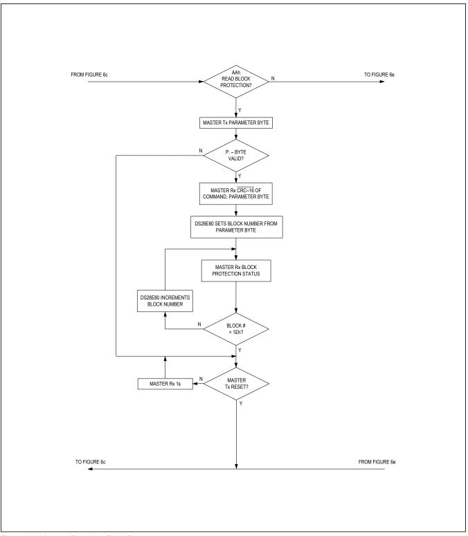
Figure 6d. Memory Functions Flow Chart
