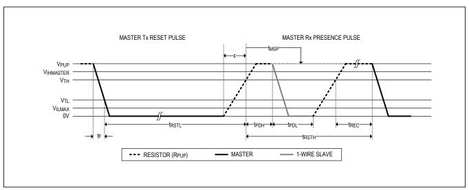
Figure 3. Initialization Procedure: Reset and Presence Pulse
