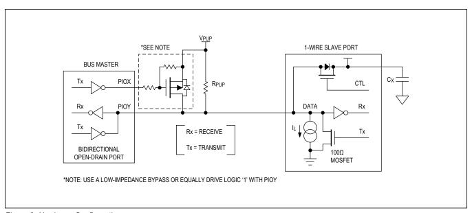
Figure 2. Hardware Configuration
