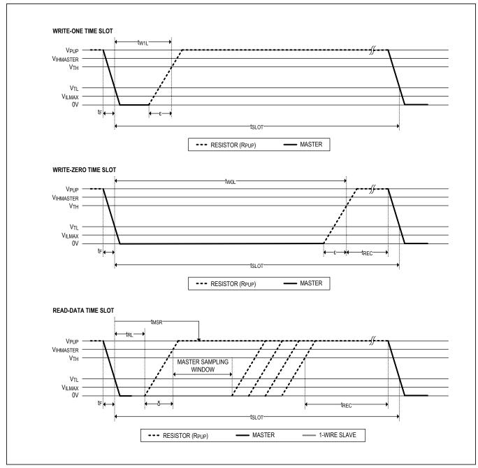
Figure 4. Read/Write Timing Diagrams
