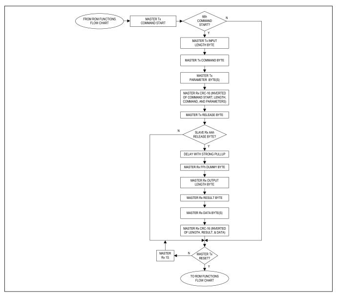
Figure 1. Device Function Flow Chart
