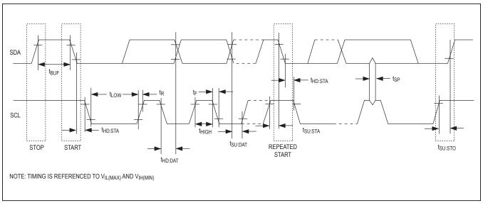
Figure 5. I<sup>2</sup>C Timing Diagram
