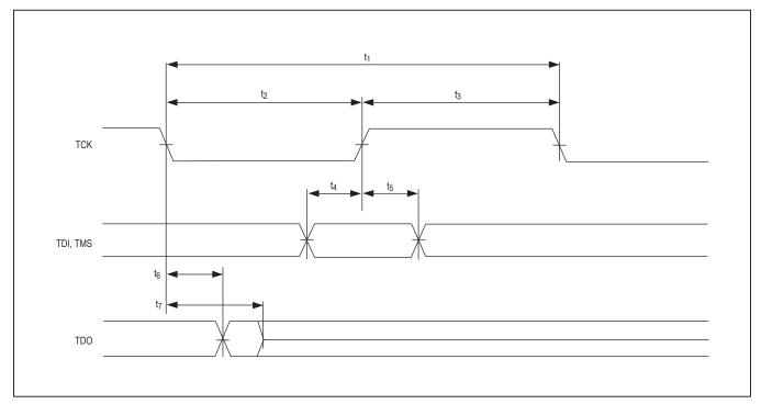
Figure 1. JTAG Timing Diagram
