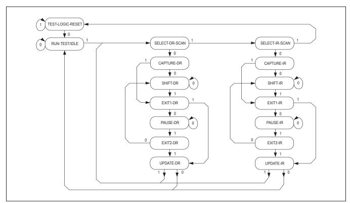
Figure 4. TAP Controller State Diagram
