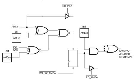
When one or more peripheral devices have been powered down due to inactivity, it may be desirable at that time to enable interrupts to at least those devices. When an access is attempted by the host, the SEM can take the appropriate action to apply power to the peripheral. During such time, the SEM can activate the  $\overline{SMI1}$  or  $\overline{SMI2}$  interrupt by writing to a power management host interface output buffer register with a status word reflecting the current condition.
