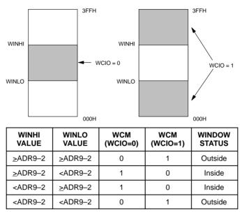
Note that there is no hardware significance to upper and lower designations. The upper comparison value can be selected as less than the lower comparison value, although doing so provides no additional function.
