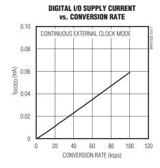
**Note 6:** For partial power-down and full power-down modes, external clock mode was used for a burst of continuous samples. Partial power-down or full power-down modes were entered thereafter. By using this method, the conversion rate was found by averaging the number of conversions over the time starting from the first conversion to the end of the partial power-down or full power-down modes.
