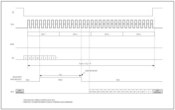
Figure 2. External Clock-Mode Conversion (Mode 0)
