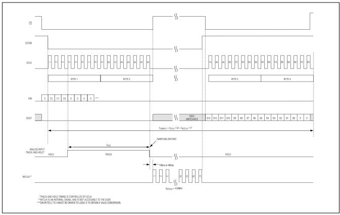
Figure 3. External Acquisition-Mode Conversion (Mode 1)
