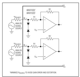
Figure 6. Simplified Analog Input Circuit
