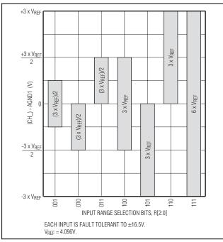
Figure 7. Single-Ended Input Voltage Ranges
