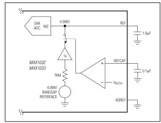
Figure 17. Internal Reference Operation
