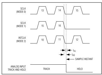
Figure 21. Aperture Diagram
