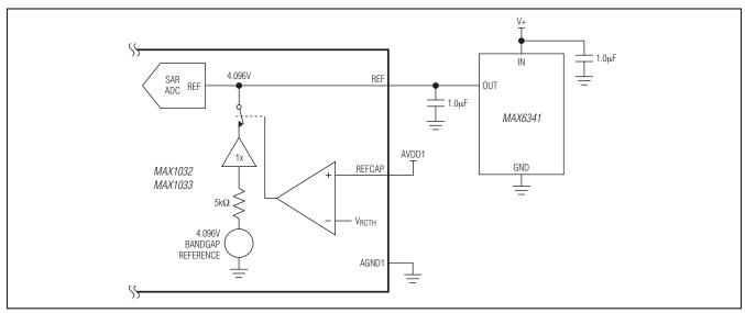
Figure 18. External Reference Operation
