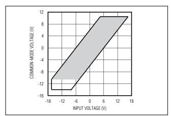
Figure 10. Common-Mode Voltage vs. Input Voltage (FSR = 6 x V<sub>REF</sub>)
