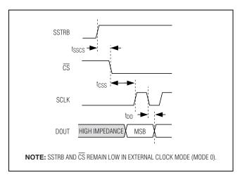
Figure 16. DOUT and SSTRB Timing
