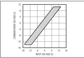
Figure 9. Common-Mode Voltage vs. Input Voltage (FSR = 3 x V<sub>REF</sub>)
