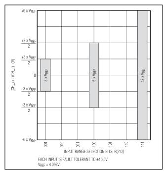
Figure 8. Differential Input Voltage Ranges
