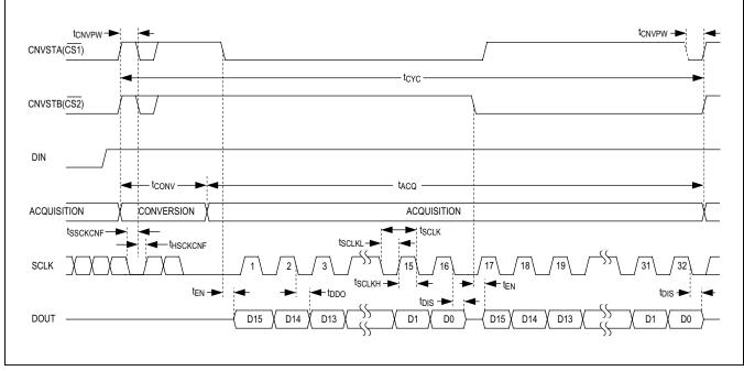
Figure 11. Multichannel CS Configuration Timing
