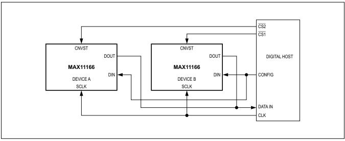
Figure 10. Multichannel CS Configuration Diagram
