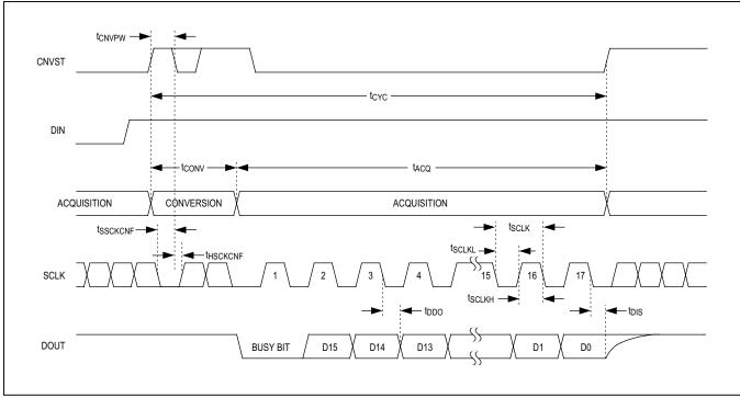
Figure 9. CS With Busy Indicator Mode Timing
