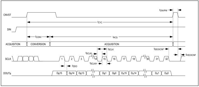
Figure 13. Daisy-Chain, No-Busy Indicator Mode Timing
