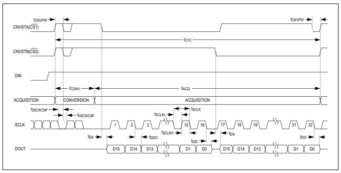
Figure 11. Multichannel CS Configuration Timing
