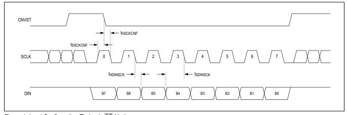
Figure 4. Input Configuration Timing in  $\overline{\text{CS}}$  Mode
