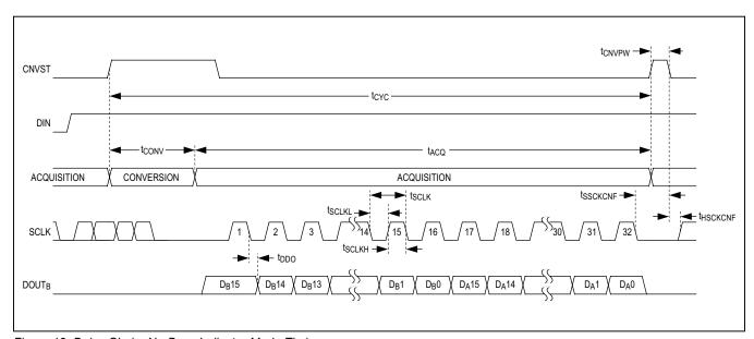
Figure 13. Daisy-Chain, No-Busy Indicator Mode Timing
