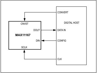
Figure 6. CS No-Busy Indicator Mode Connection Diagram
