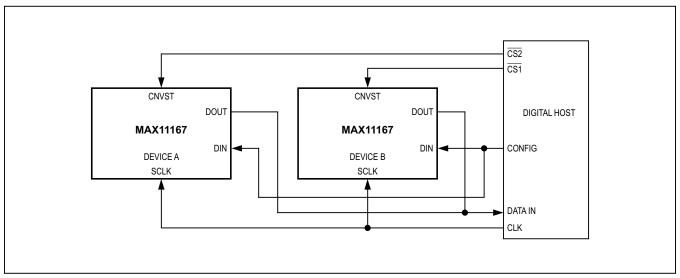
Figure 10. Multichannel CS Configuration Diagram
