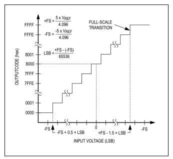
Figure 3. Bipolar Transfer Function
