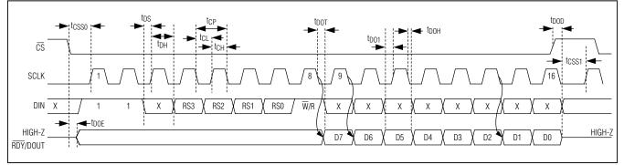
Figure 7. SPI Register Access Read
