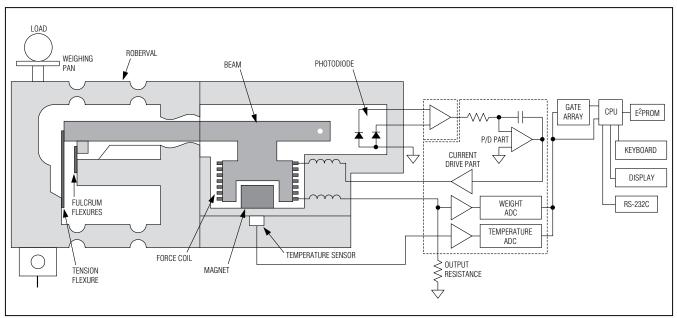
Figure 10. Typical Magnetic Force Restoration Scale
