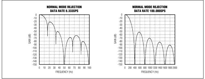
Figure 2. Normal-Mode Frequency Response (2.048MHz Oscillator, LINEF = 1)
