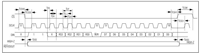
Figure 6. SPI Register Access Write
