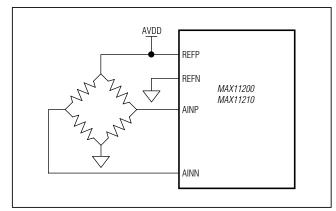
Figure 9. Resistive Bridge Measurement Circuit
