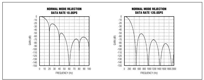
Figure 1. Normal-Mode Frequency Response (2.4576MHz Oscillator, LINEF = 0)
