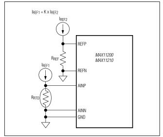
Figure 8. RTD Temperature Measurement Circuit
