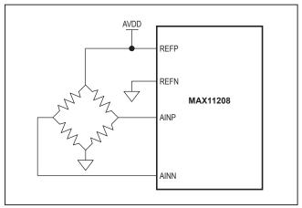
Figure 7. Resistive Bridge Measurement Circuit
