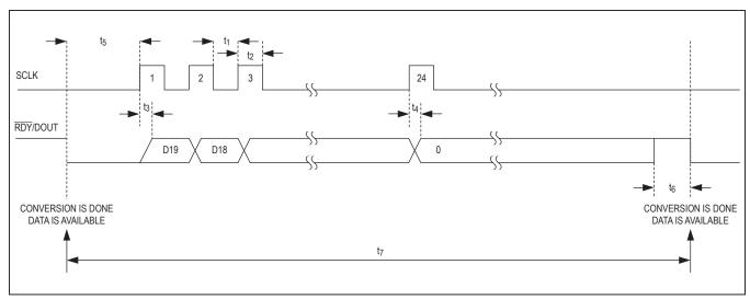
Figure 1. Timing Diagram for Data Read After Conversion
