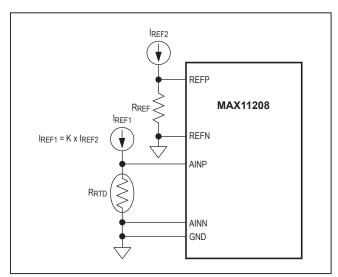
Figure 6. RTD Temperature Measurement Circuit
