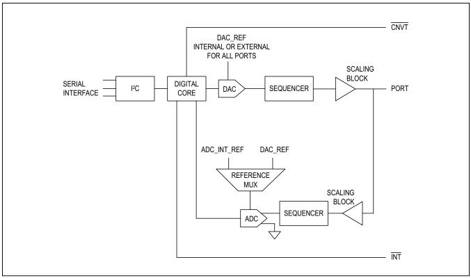
Figure 6. DAC Configuration with ADC Monitoring
