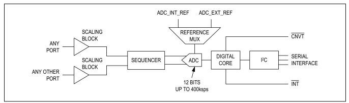
Figure 3. ADC with Differential Inputs
