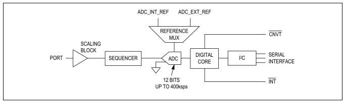
Figure 2. ADC with Single-Ended Input
