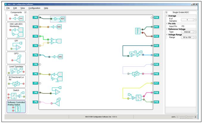
Figure 13. Example of GUI to Develop Configuration File
