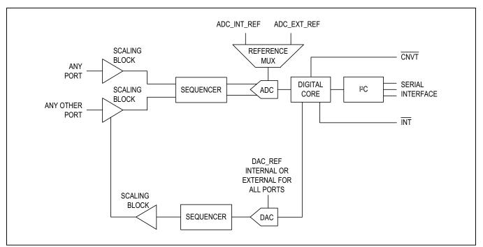
Figure 4. ADC with Pseudo-Differential Input Set by DAC
