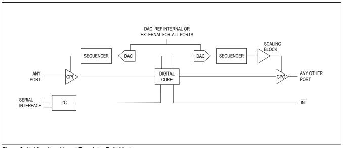
Figure 9. Unidirectional Level Translator Path Mode
