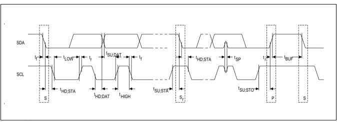
Figure 1. I<sup>2</sup>C Timing
