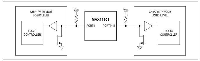
Figure 10. Bidirectional Level Translation Application Diagram
