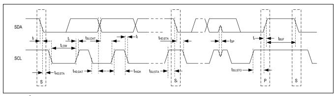
Figure 1. I<sup>2</sup>C Timing
