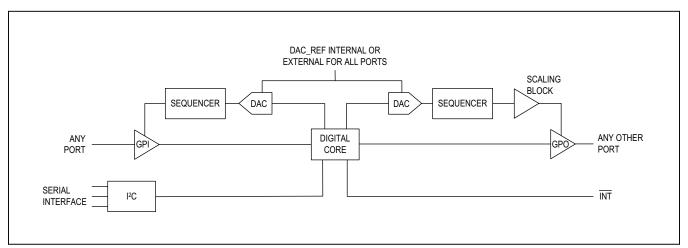
Figure 9. Unidirectional Level Translator Path Mode
