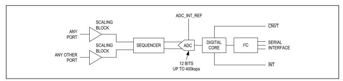
Figure 3. ADC with Differential Inputs
