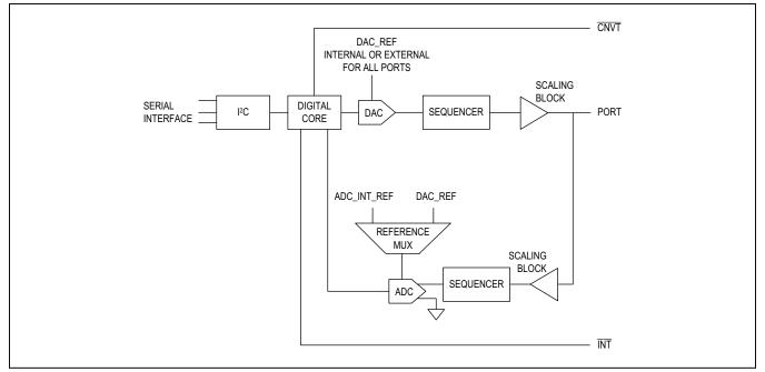
Figure 6. DAC Configuration with ADC Monitoring
