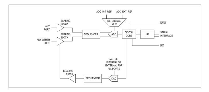
Figure 4. ADC with Pseudo-Differential Input Set by DAC
