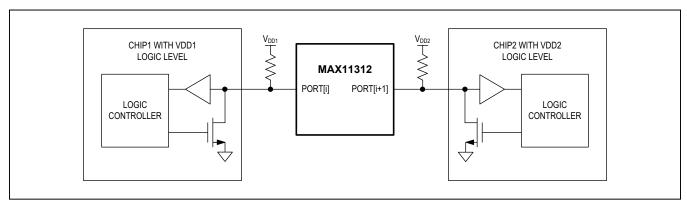
Figure 10. Bidirectional Level Translation Application Diagram
