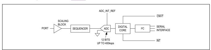
Figure 2. ADC with Single-Ended Input
