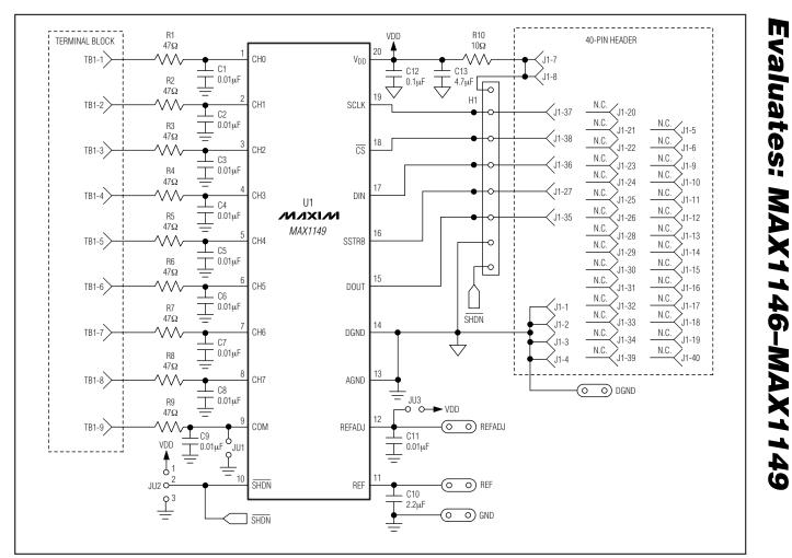
Figure 2. MAX1149 EV Kit Schematic
