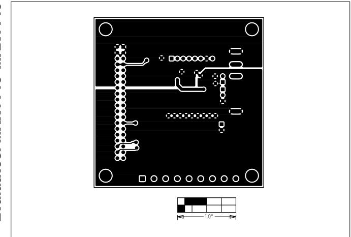
Figure 5. MAX1149 EV Kit PC Board Layout—Solder Side
