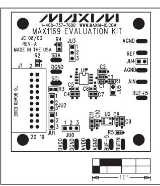
Figure 3. MAX1169 EV Kit Component Placement Guide— Component Side
