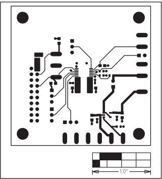
Figure 4. MAX1169 EV Kit PCB Layout—Component Side
