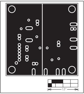
Figure 5. MAX1169 EV Kit PCB Layout—Inner Layer 2 (GND)
