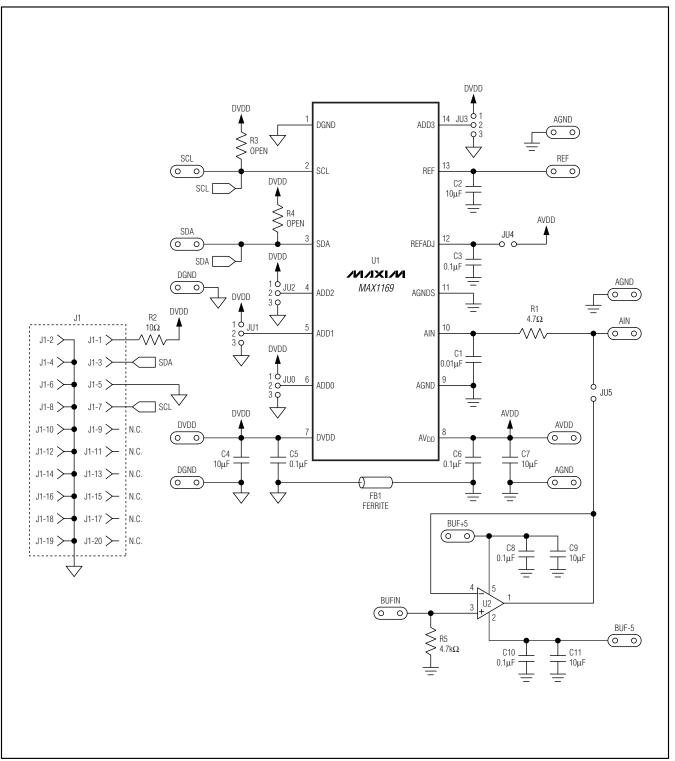
Figure 2. MAX1169EV Kit Schematic
