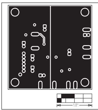
Figure 7. MAX1169 EV Kit PCB Layout—Solder Side
