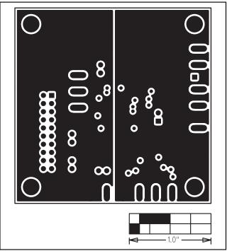
Figure 6. MAX1169 EV Kit PCB Layout—Inner Layer 3 (VDD)
