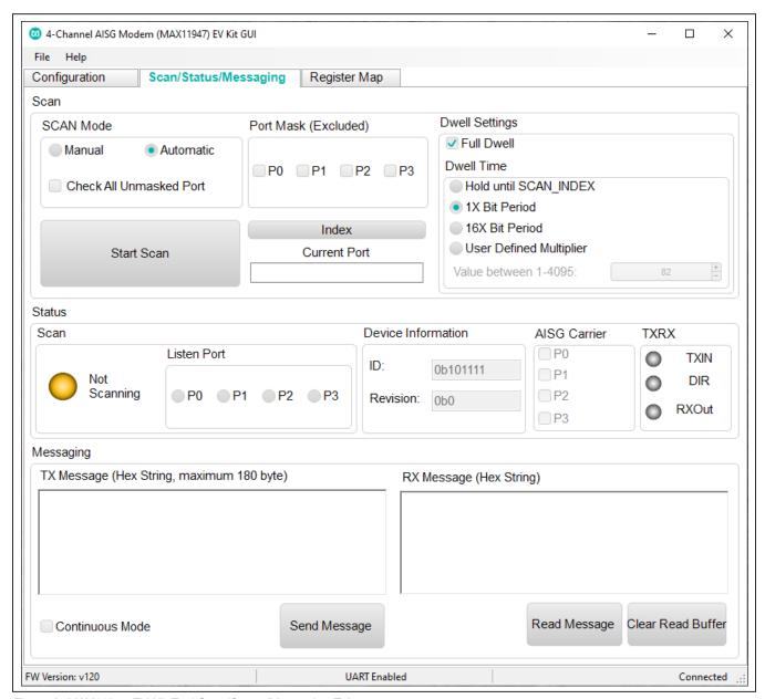
Figure 8. MAX11947 EV Kit Tool Scan/Status/Messaging Tab
