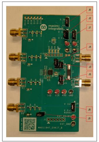
Figure 2. MAX11947 EV Kit Board—Jumper Locations
