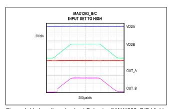
Figure 4. Undervoltage Lockout Behavior (MAX1293\_B/C High)
