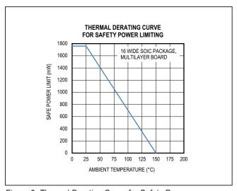
Figure 2. Thermal Derating Curve for Safety Power Limiting—16 Wide SOIC
