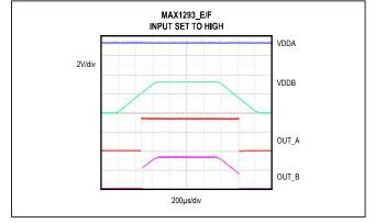
Figure 6. Undervoltage Lockout Behavior (MAX1293\_E/F High)
