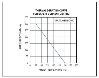
Figure 3. Thermal Derating Curve for Safety Current Limiting
