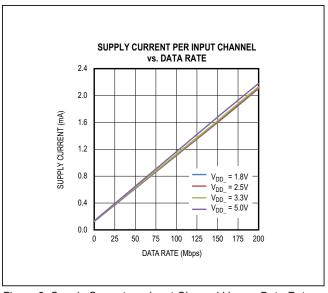
Figure 8. Supply Current per Input Channel Versus Data Rate
