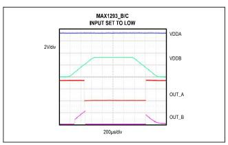
Figure 5. Undervoltage Lockout Behavior (MAX1293\_B/C Low)
