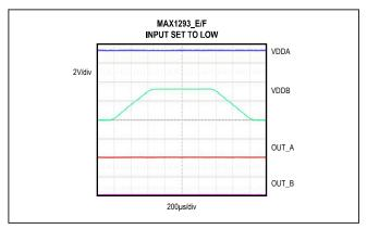
Figure 7. Undervoltage Lockout Behavior (MAX1293\_E/F Low)
