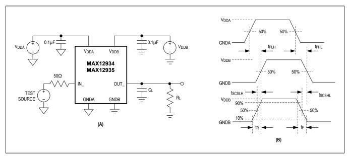
Figure 1. Test Circuit (A) and Timing Diagram (B)
