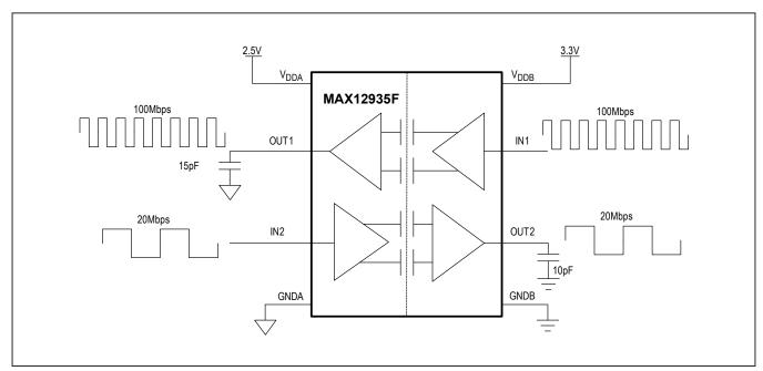
Figure 10. Example Circuit for Supply Current Calculation
