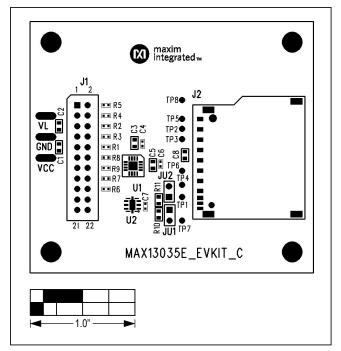
Figure 2. MAX13035E EV Kit Component Placement Guide—Component Side
