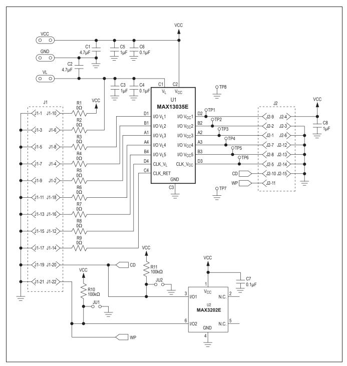
Figure 1. MAX13035E EV Kit Schematic
