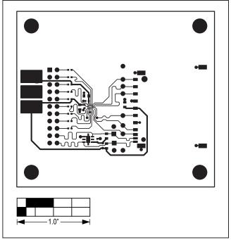
Figure 3. MAX13035E EV Kit PCB Layout—Component Side
