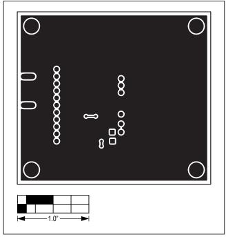
Figure 4. MAX13035E EV Kit PCB Layout—Solder Side
