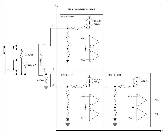
Figure 12. Diagnostic Setup for Remote Jack Sense
