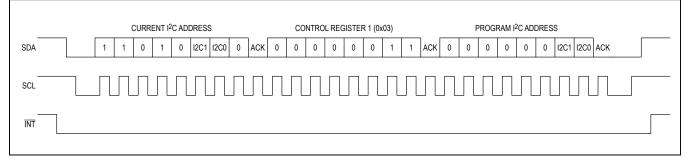
Figure 6. I<sup>2</sup>C Slave Address Programming
