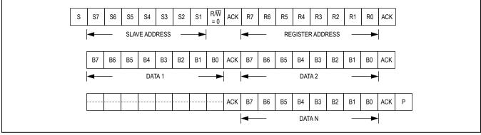
Figure 8. A Burst-Write Operation
