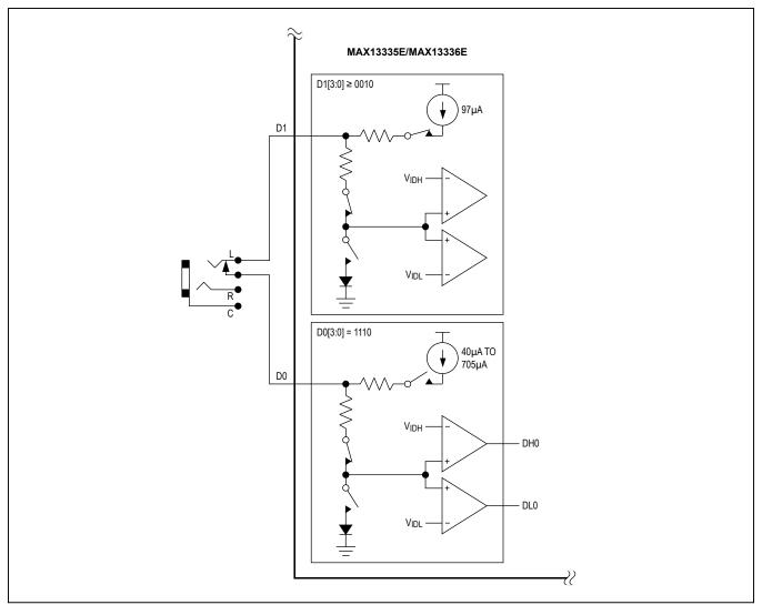
Figure 11. Diagnostic Setup for Local Jack Sense
