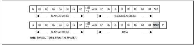
Figure 9. A Single Byte-Read Operation
