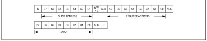
Figure 7. A Single Byte-Write Operation
