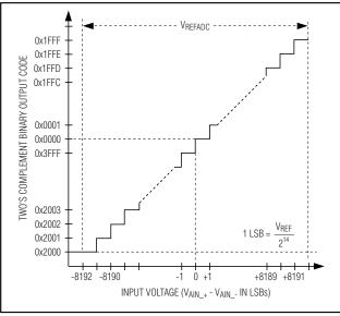
Figure 11. ±1.25V Transfer Function
