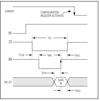
Figure 4. Write Timing
