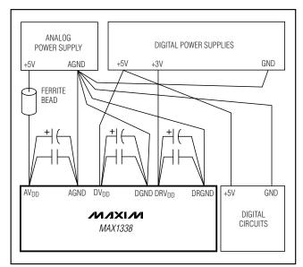
Figure 12. Power-Supply Grounding and Bypassing
