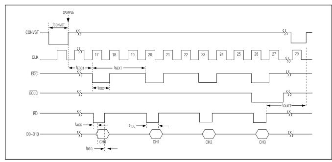
Figure 5. Reading During a Conversion—Internal or External Clock
