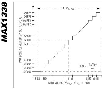
Figure 9. ±5V Transfer Function
