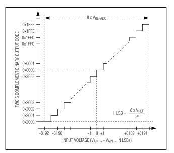
Figure 8. ±10V Transfer Function
