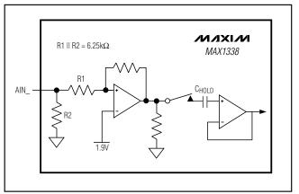
Figure 3. Simplified Typical Input Circuit
