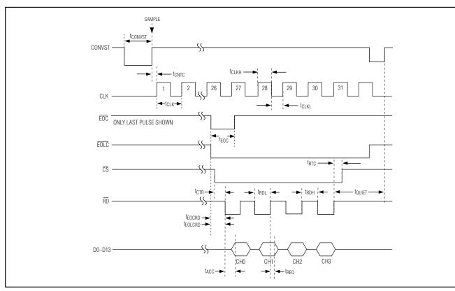
Figure 6. Reading After a Conversion—External Clock
