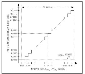
Figure 10. ±2.5V Transfer Function
