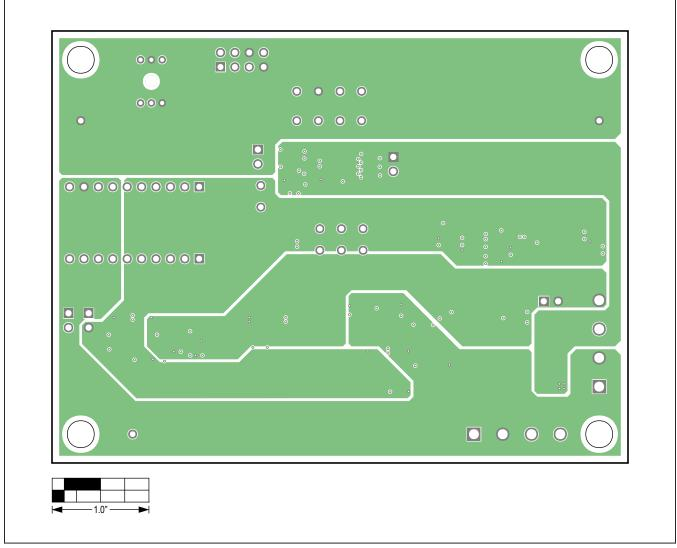
MAX1452 EV System PCB Layout Diagram—Internal 3
