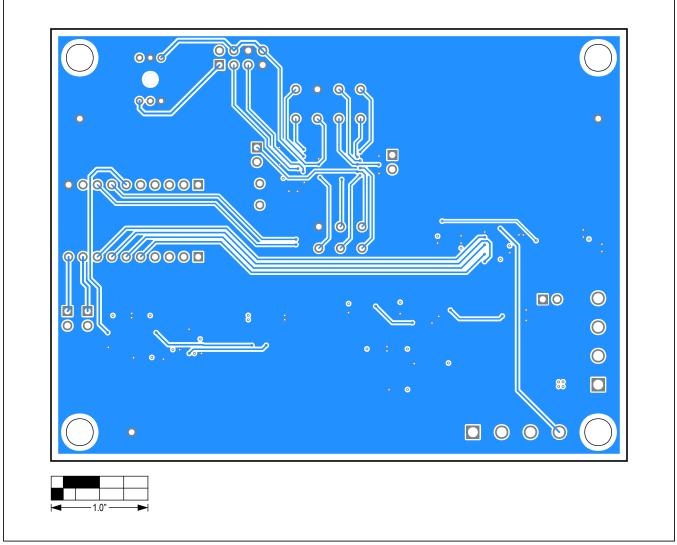
MAX1452 EV System PCB Layout Diagram—Bottom Layer
