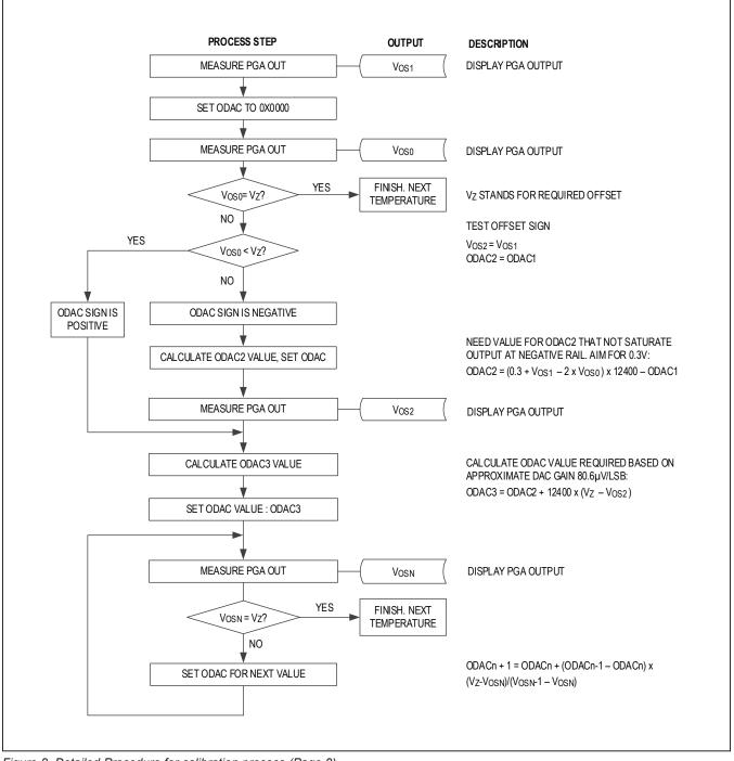
Figure 8. Detailed Procedure for calibration process (Page 2)
