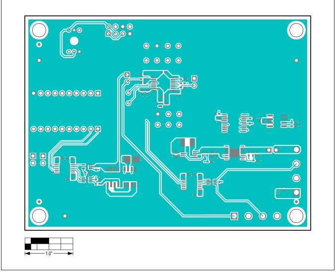
MAX1452 EV System PCB Layout Diagram—Top Layer
