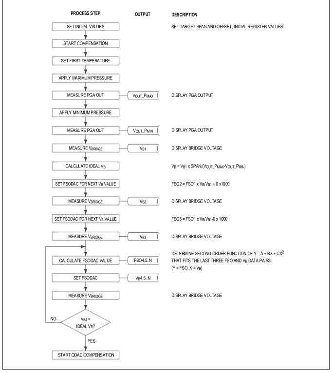
Figure 7. Detailed Procedure for calibration process (Page 1)
