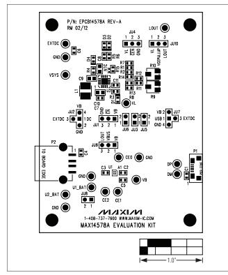
Figure 2. MAX14578A EV Kit Component Placement Guide— Component Side
