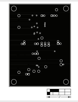
Figure 4. MAX14578A EV Kit PCB Layout—Ground Layer 2
