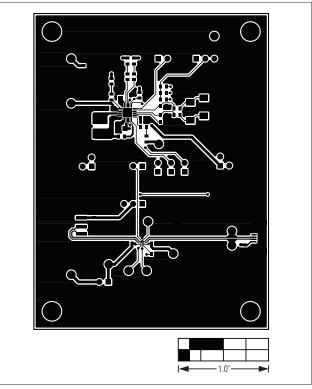
Figure 3. MAX14578A EV Kit PCB Layout—Component Side
