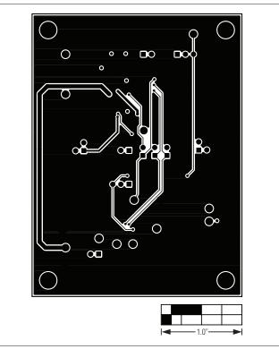
Figure 6. MAX14578A EV Kit PCB Layout—Solder Side
