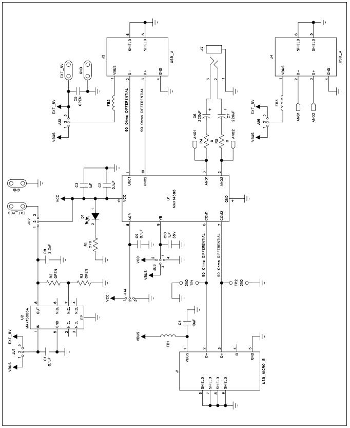
Figure 1. MAX14585 EV Kit Schematic
