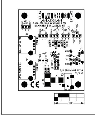
Figure 2. MAX14585 EV Kit Component Placement Guide— Component Side
