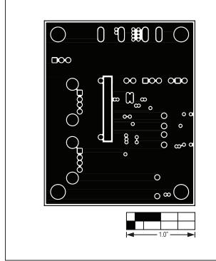
Figure 5. MAX14585 EV Kit PCB Layout—Inner Layer 3
