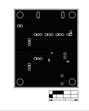
Figure 4. MAX14585 EV Kit PCB Layout—Inner Layer 2
