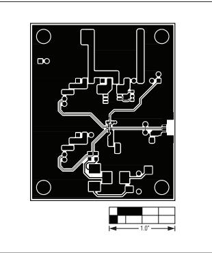
Figure 3. MAX14585 EV Kit PCB Layout—Component Side
