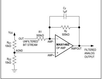
Figure 8. Filtering the Output DAC
