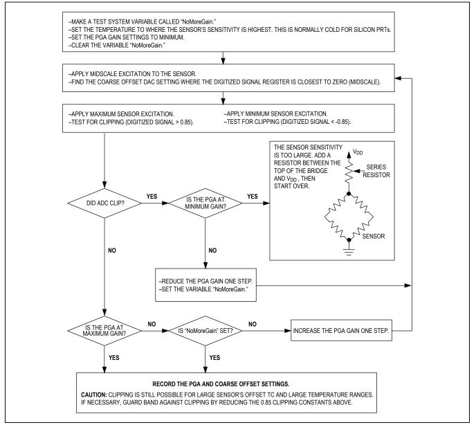
Figure 1. Flowchart for Determining PGA and CO Settings
