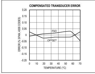
Figure 7. Compensated Sensor/MAX1462 Pair
