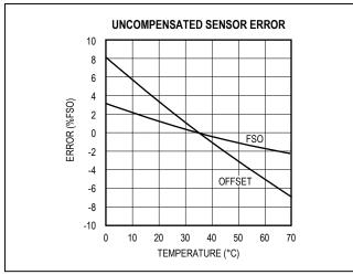
Figure 6. Sensor Characteristics Before Compensation
