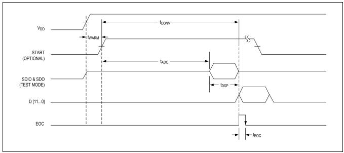
Figure 5. MAX1462 Conversion Timing
