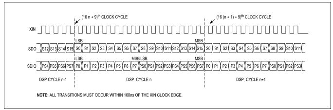
Figure 4. DSP Serial Output Timing Diagram
