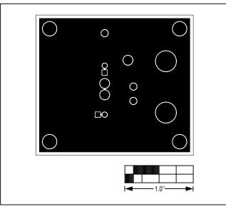
Figure 4. MAX14653–MAX14655 EV Kit PCB Layout— Solder Side
