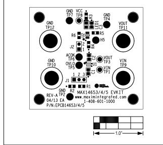
Figure 2. MAX14653–MAX14655 EV Kit Component Placement Guide—Component Side
