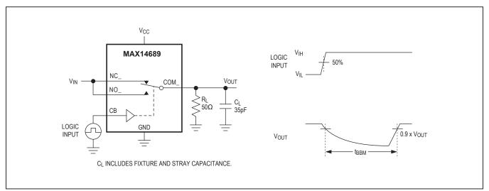
Figure 2. Break-Before-Make Interval
