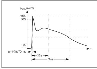
Figure 7. IEC 61000-4-2 ESD Generator Current Waveform
