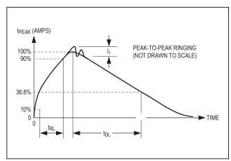
Figure 5. Human Body Current Waveform
