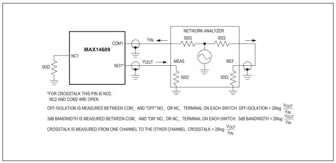
Figure 3. 3dB Bandwidth, Off-Isolation, and Crosstalk
