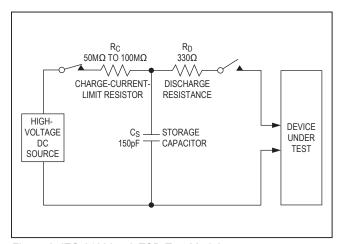
Figure 6. IEC 61000-4-2 ESD Test Model
