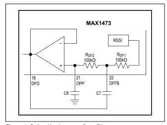
Figure 1. Sallen-Key Lowpass Data Filter
