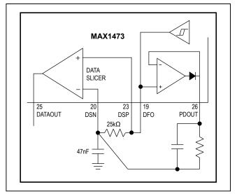
Figure 4. Using PDOUT for Faster Startup
