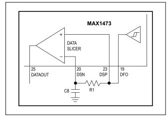
Figure 2. Generating Data Slicer Threshold
